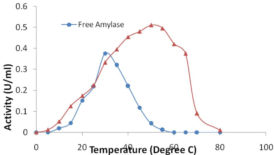
Fig 2: Effect of temperature on the activity of soluble and immobilized amylase.
