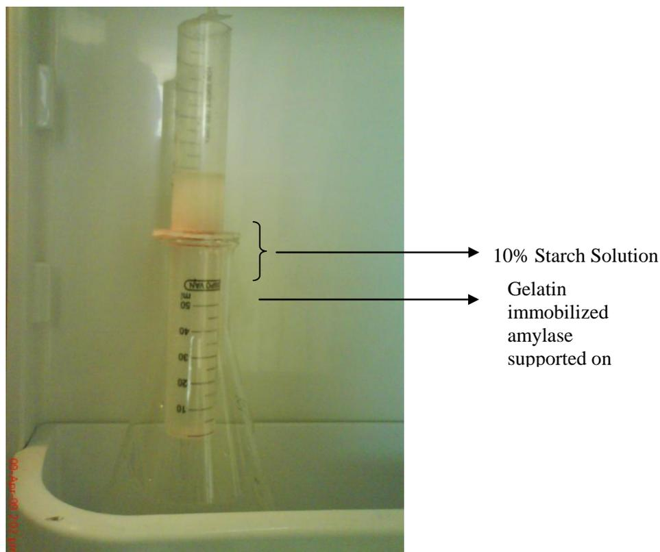
**Fig.5. Column for the production of glucose from starch by gelatin immobilized amylase. The upper syringe contain 10% starch solution which is converted by immobilized amylase, placed in the mid of column supported by a nylon cloth. The hydrolyzed product is collected in the lower column.**
